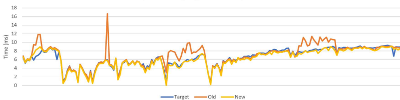
Old and new asynch algorithms overlaid onto LVDT data
